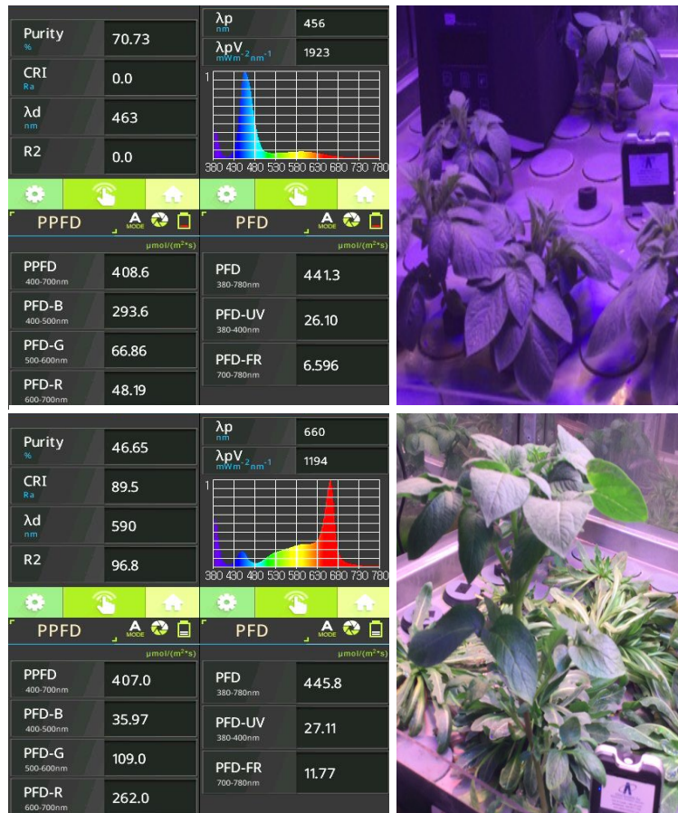
Fig. 1. Spectral characteristics of phytotron chambers. PAR+BL (blue light, above): total photon flux is
